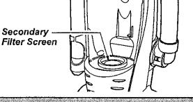
The secondary filter screen protects the motor.
